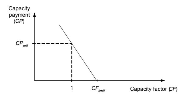
Capacity factor, *CF* = Available capacity/peak load
